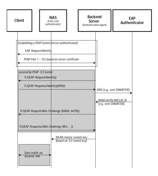
Figure 3: PEAP with EAP AKA: Example Message Flow
