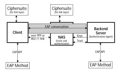
Figure 2: Relationship between EAP client, back-end authentication server and NAS in PEAP [3]
