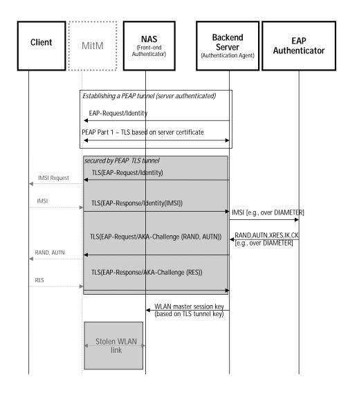
Figure 4: Man-in-the-Middle in PEAP, e.g., with EAP AKA
